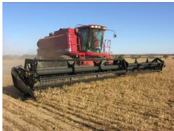
Fig. 4. Finger tine reel on a draper front.
