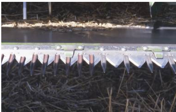
Fig. 1. Double density (quad) knife and single density single density knife sections.
