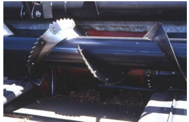
Fig. 7. Lupin Breakers® fitted to the centre auger on a draper front.
