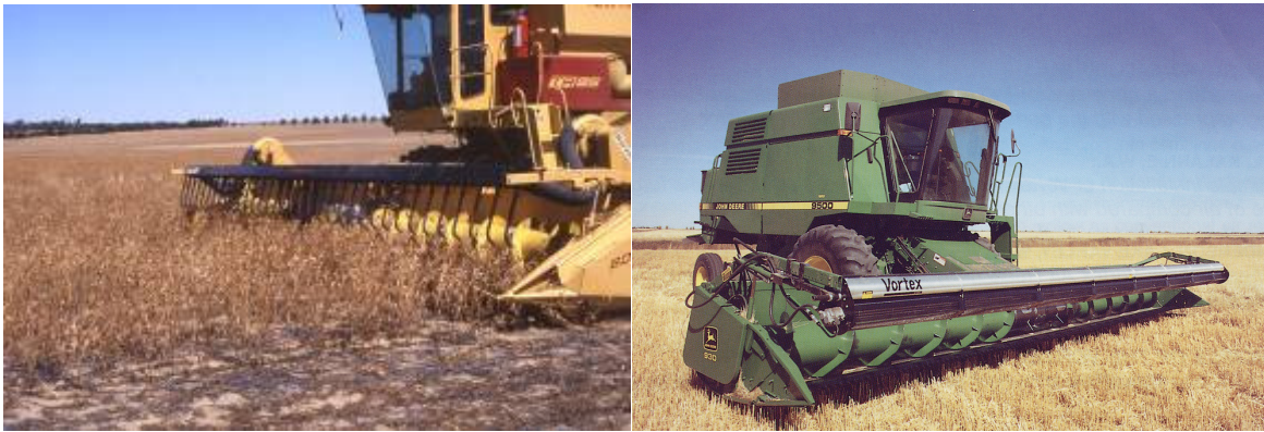
Fig. 5. Manifold air reel on a conventional auger front (left) and a full width fan (right).
