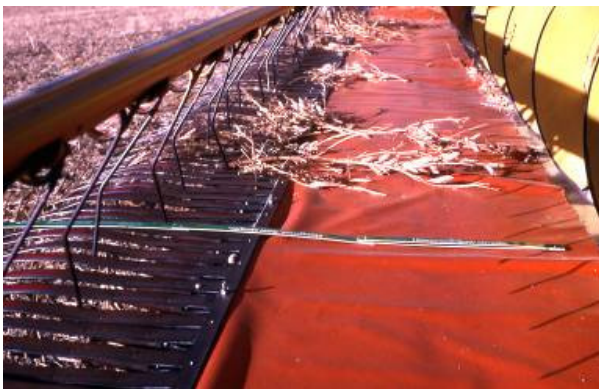
Fig. 6. Vibra-Mat® attached to the knife back.
