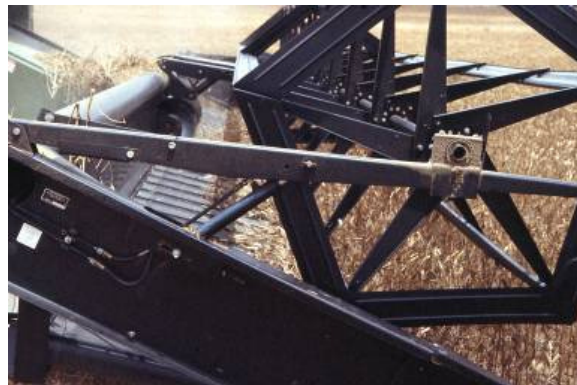
Fig. 3. Batt reel on a draper type front.
