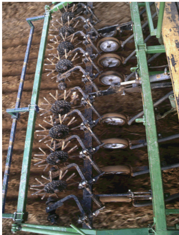
Fig. 1. Lupin seed pressed into the soil (top photo) before covering with loose soil by a rotary harrow with depth gauge wheels on the ends (bottom photo).
