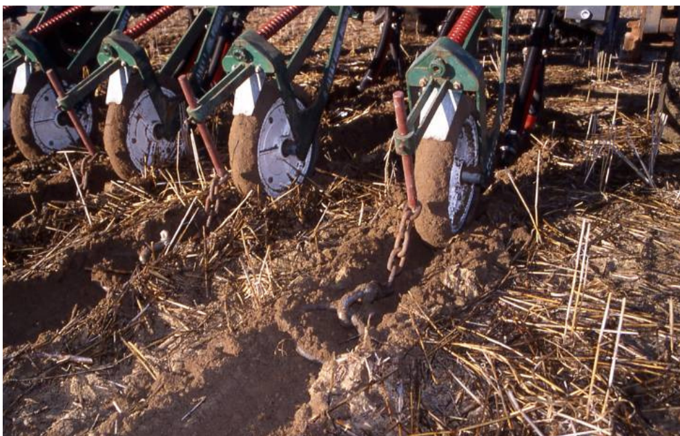
Fig. 2. A ring harrow following press wheels to bring loose soil over the seed.
